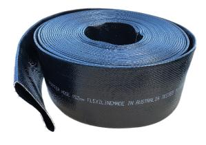
Flexiline™ is a flexible layflat hose used for industrial pumping applications. It is robust and typically used for pumping pressures operating up to 1500 kPa. It can be supplied with a large range of couplings, including Bauer, for quick-connect dewatering use. Lengths up to 20 m can be easily handled. However, for longer lengths, we recommend our reel systems; this makes the handling safe, quick and easy.
