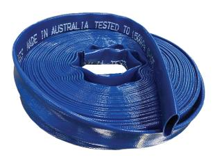
Aqualine™ is a high-quality layflat hose for use with potable water. It is manufactured by weaving a textile reinforcement of high-tensile polyester and extruded with potable water-approved polyurethane. This flexible hose also has good resistance to abrasion and can withstand moderate traffic.
