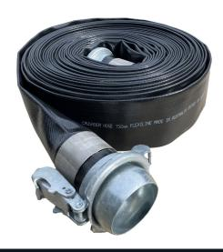
**Flexiline** is a flexible layflat hose used for industrial pumping applications. It is robust and typically used for pumping pressures operating up to 1500 kPa. It can be supplied with a large range of couplings, including Bauer for quick-connect dewatering use. Lengths up to 20 m can be easily handled. However, for longer lengths we recommend our reel systems; this makes the handling safe, quick and easy.
