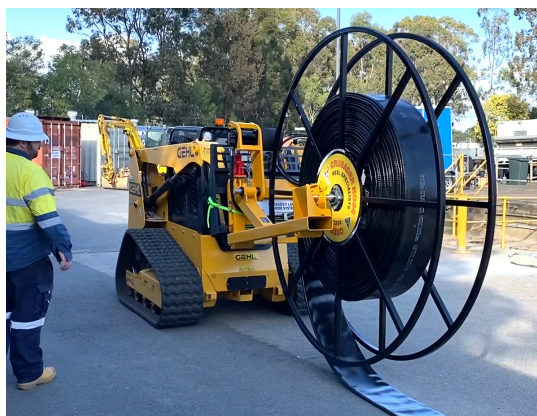
The Hamersley Reel System deploying 200 m of Waterlord layflat hose
