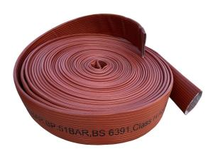
Fortex is an extruded rubber hose for professional firefighting applications. It is made by weaving high-tenacity yarns and covering the textile reinforcement with a synthetic rubber compound. This process creates a high-pressure fire hose that is abrasion and chemical resistant.
