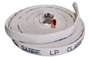
**Sabre** is a percolating hose which allows water to seep through the textile reinforcement. By mechanically pin pricking the hose over its length, a thin water layer forms over the hose offering extra protection against burning coals.
