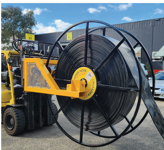
The Hamersley Reel System deploying 200 m of Waterlord layflat hose
